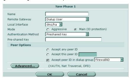
Figure 19: Configure VPN IPSec dialup authentication
